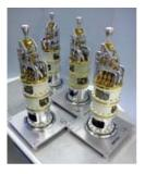
before it is delivered to the ALMA Back-End System. The SIS detector and the HEMT IF amplifier must operate at a cryogenic temperature of 4 Kelvin. NRC-HIA has developed a cryogenic 4-8 GHz HEMT amplifier for this application.
